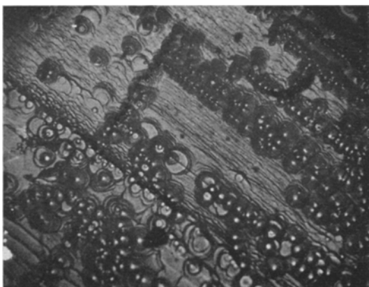
Figure 2 Pile up of non-basal screw dislocations along crystal ledges ( \times 140 ).
