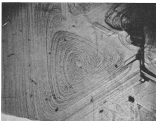
Figure 4 Growth hill showing curved spiral arms ( \times 140 ).
