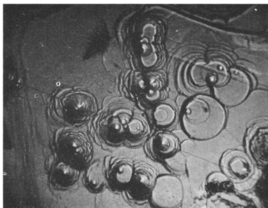
Figure 1 Characteristic etch pattern on GaSe (0001) surface using diluted chromic-sulphuric acid as etchant ( \times 140 ).
